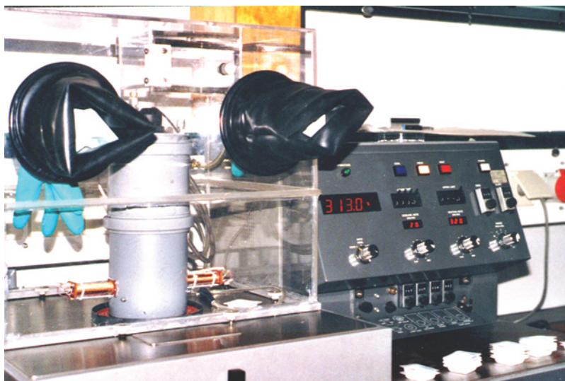
Figure 3. Photograph of the modified head of the photo-DSC, which makes it possible to measure the heat of photochemical reactions. The vertical tube to the left contains the light source and a computer controlled optical shutter for irradiation of the sample. The glove box is needed to investigate radical reactions in an oxygen-free environment. (Figure appears in color online.)
